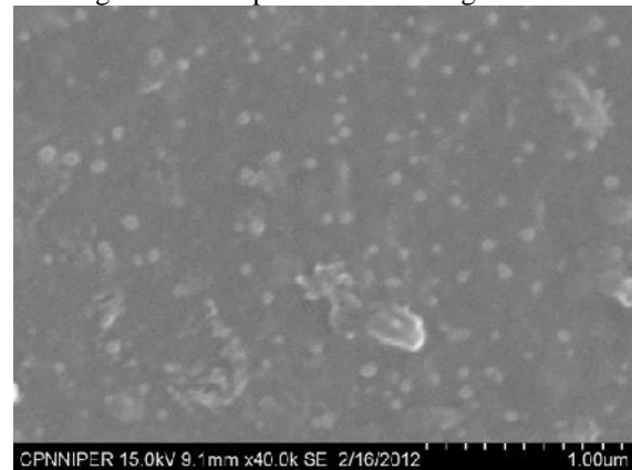
Fig. 7: SEM image of PtNPs synthesized by CFE of S. boulardii
